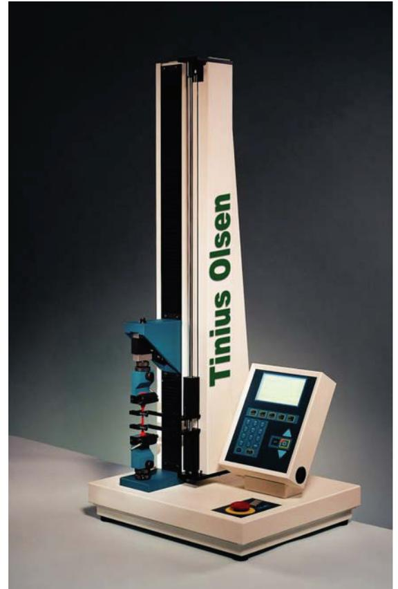
**Fig 3.** Model H5kS testing machine with 100 RC long travel extensometer.
